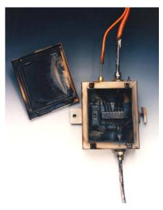
On the successful conclusion of this test, which is designated "fire-alone" BS6387'C', the next test is to mount the sample (still powered-up) on a flat vertical surface and to apply flame at a temperature of 950°C (1742°F) (by means of a flame gun) whist at the same time striking the board on which the sample is mounted with a 25mm (1") diameter iron bar every 30 seconds for a period of 15 minutes. This is designated the "impact test" BS6387'Z'.
