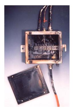
SX Range Enclosure and Cables after IEC331 Fire Testing
