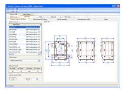
Some years ago we decided to make this program available to all our customers, free of charge, and this has been a tremendous success. The software allows users to easily design complex arrangements of entries and generates a drawing which ABTECH can subsequently use for manufacturing purposes.
