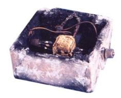
Due to the enclosure's labyrinth seal system, whereby the seal is protected from external forces, the BPG range has excellent ingress protection qualities which mean that the enclosures are tested to and passed IP66/67. They have also undergone and passed the Shell/ERA deluge test which was devised to adequately test enclosures and electrical equipment which is routinely subjected to ship decks conditions or fire deluge systems.
