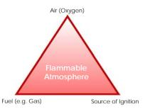
With this knowledge, it is possible to protect the equipment from one of the three elements required to cause an explosion i.e. in the case of increased safety (EEx'e') the ignition source is removed by ensuring that there are no hot surfaces or sparking components which could ignite a fuel and oxygen mixture which may enter the enclosure.
