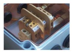
Each enclosure comes pre-drilled with four M20 tapped cable entries and is supplied with certified blanking plugs. The BPGA range of enclosures are ATEX and IECEx certified Ex'e' and are suitable for use in Category 2/Zone 1 & 21 and Category 3/Zone 2 & 22 areas according to EN 60079-14.
