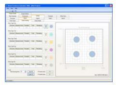
The program also incorporates a terminal calculation program which lets you see at a glance whether or not the desired number of terminals can be accommodated within your chosen enclosure and as with the Entry Calculator will print a drawing of your finished design.
