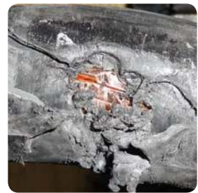
Major cable damage caused by thread contact
