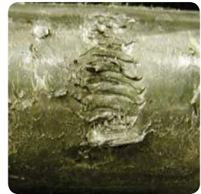
Minor cable damage caused by thread contact
